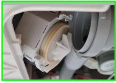
4) Check the connector connection to the <u>drain pump (photo 1) & wash pump (photo 2)</u> whether the connector is fastened entirely inside the socket (according to the photo below). Push the connector to the end of the socket. If after pushing you hear distinctive "click" it means that the connector was not fastened properly.
