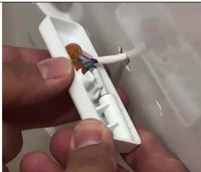
6. Fit the new sensor in the cover of the housing and fit the cable as shown in the figure.
